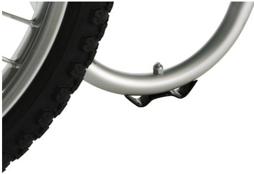
Installed skid plate
